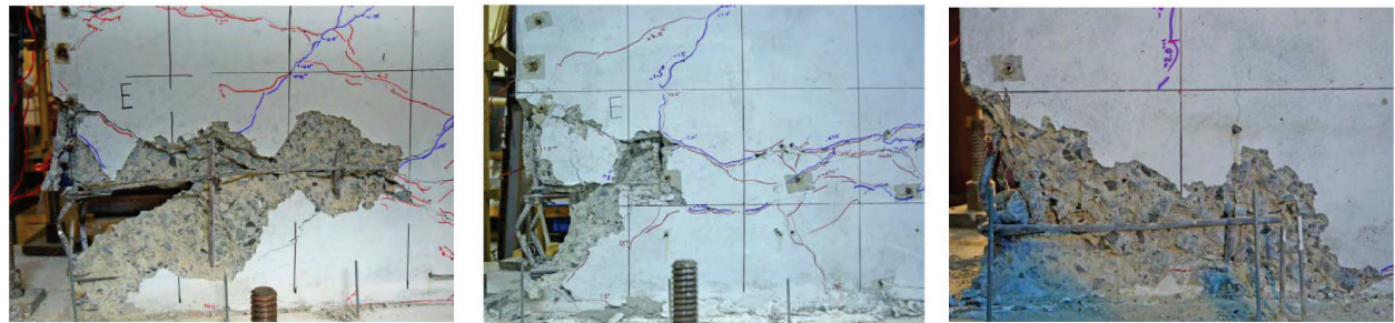
Figure 8-23 Measured hysteretic response and toe damage at end of each test for Specimens C1, C2, and C3 (from Lu et al., 2017).
