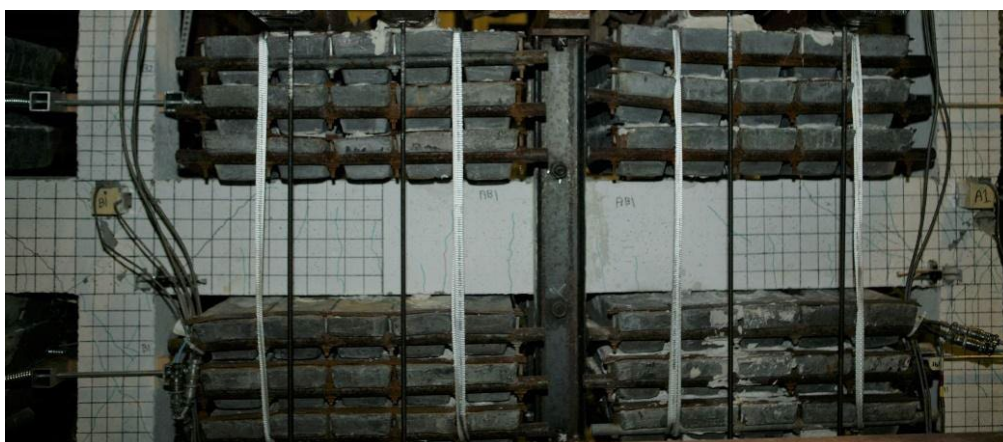
Figure 3-20 Column B1 (left) and column A1 (right) observations after Dynamic Test 1 at Level 1.
