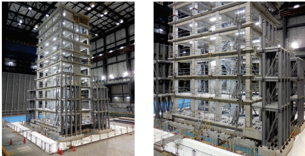
Figure 5-1 10-story structure tested at E-Defense shake table in 2015 (photo courtesy of J. Wallace).
