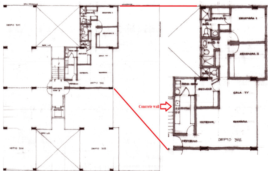
Figure 10-28 Masonry wall and infill wall locations for an apartment unit of a typical floor.
