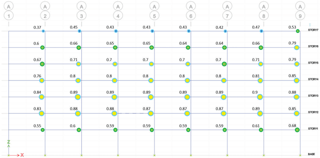
Figure C-25 AR Beam Negative Moment, ASCE 41: BSE-2N - Soil Takes Tension (CP)
