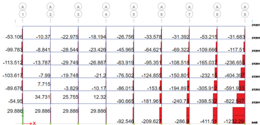
Figure C-20 Column Axial Load, LC - 0.9D + E (BSE-2N) Soil no Tension, k_{sv} = 0.1 kci,
